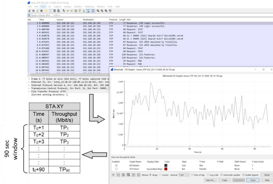
Figure 11: Derivation of throughput statistics from Wireshark software traces.
